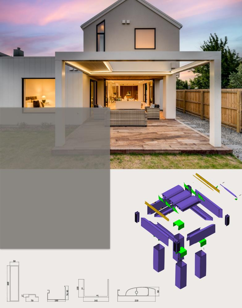
Aluminium grade - 6063T6 304/316 Stainless steel fasteners
